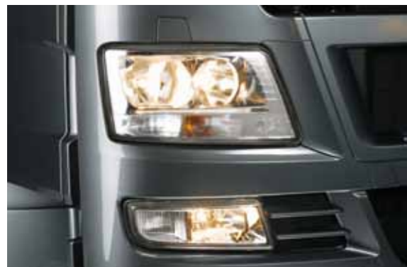
Headlights with free-form reflectors, Xenon dipped light.
