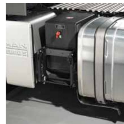
Compact battery box.
