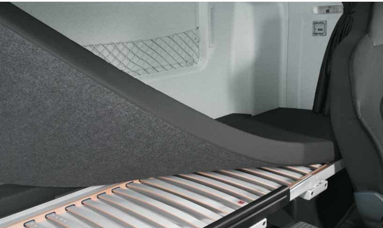
Bunk with a slatted frame and cold foam mattress.
