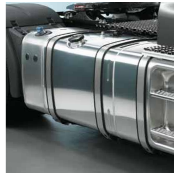
Combination tank for diesel and AdBlue®.
