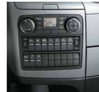
Controls for the air-conditioner, heater and ventilation. Switch panel with function displays.
