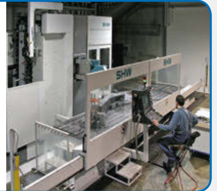
Flatbed milling machine in plant I
