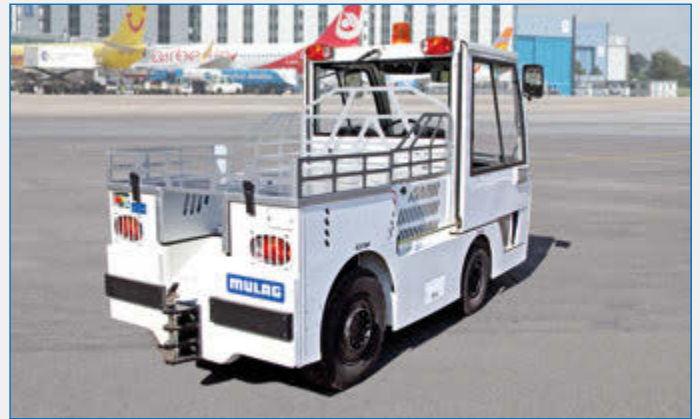
Comet 3 FC prototype with innovative hydrogen fuel cell drive
